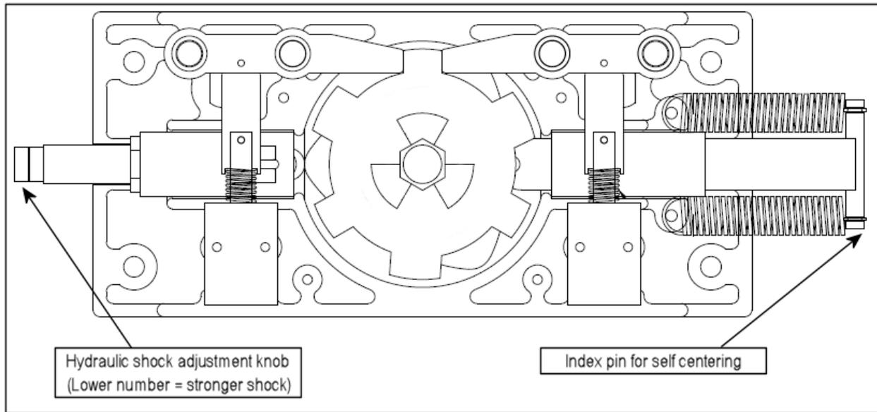
Should the shock need replaced, be sure not to fully thread the shock into the shock housing. Instead, thread the shock until it no longer spins, and then back the shock out approximately 1 ½ - 2 turns until the set screw is facing up. Lock down the shock with the provided nut, and then make field adjustments to the shock strength.
