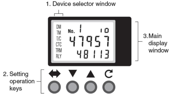
Although the logic controller is capable of many functions, all of the devices that the control head operates from are accessed in “Device Mode”. When device mode is active, the display screen will show DM in the top left corner.
