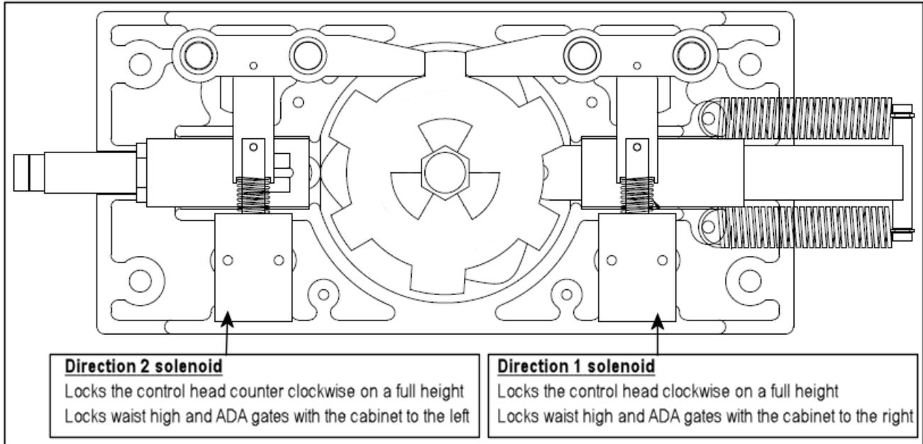
If removing the locking bar becomes necessary for any reason, two methods can be used. The easiest method is to punch the 1/2" dowel pin out from the bottom side of the control head. This releases the locking bar from the casting. An alternate approach would be to remove the (4) 1/4-20 socket head cap screws from the casting and remove the lid.
