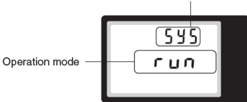
Although under normal circumstances you should never encounter this window, if by accident you should happen to come across it, simply press the up or down arrow until the window reads “run”. Press and hold the **C** button for 3 seconds, and the display will return to device mode.
