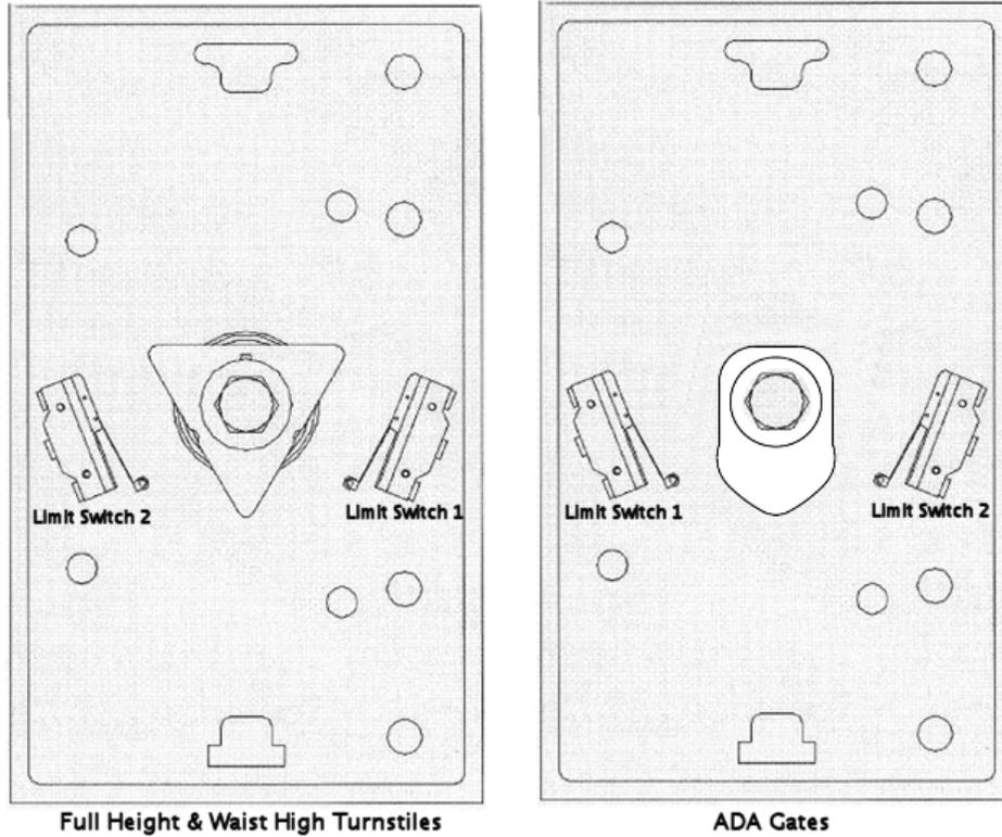
*Note: When replacing a switch, be sure to utilize the normally open and common screw terminals. Normally open should go into the PLC's Limit Inputs and Common should go to 24VDC+*
