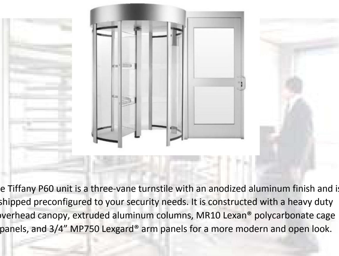
The Tiffany P60 unit is a three-vane turnstile with an anodized aluminum finish and is shipped preconfigured to your security needs. It is constructed with a heavy duty overhead canopy, extruded aluminum columns, MR10 Lexan® polycarbonate cage panels, and 3/4" MP750 Lexgard® arm panels for a more modern and open look.
